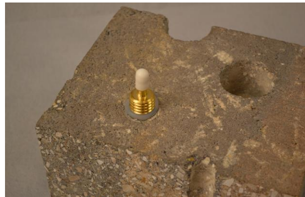
Figure 3. Installed VAPOR PIN®
