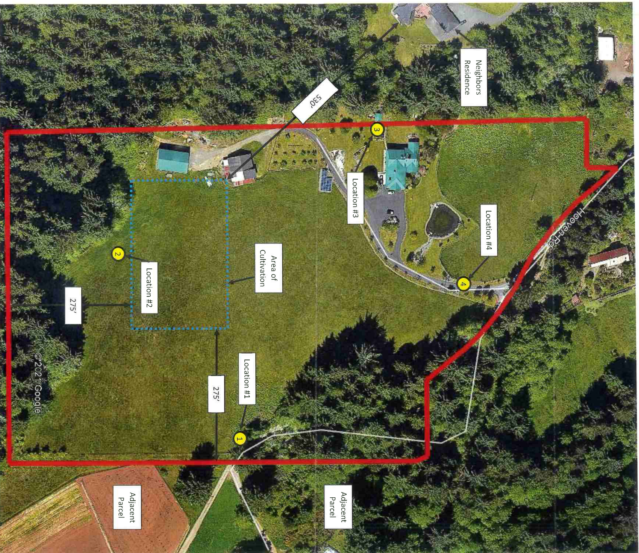
Figure 1: Property Diagram with associated Location of the four (4) noise testing sites, area of cultivation, neighboring residences and parcels, and setbacks to cultivation.
