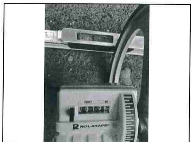
Photo #18 Cobb Rd Slope 15.1% Width 13'2"
