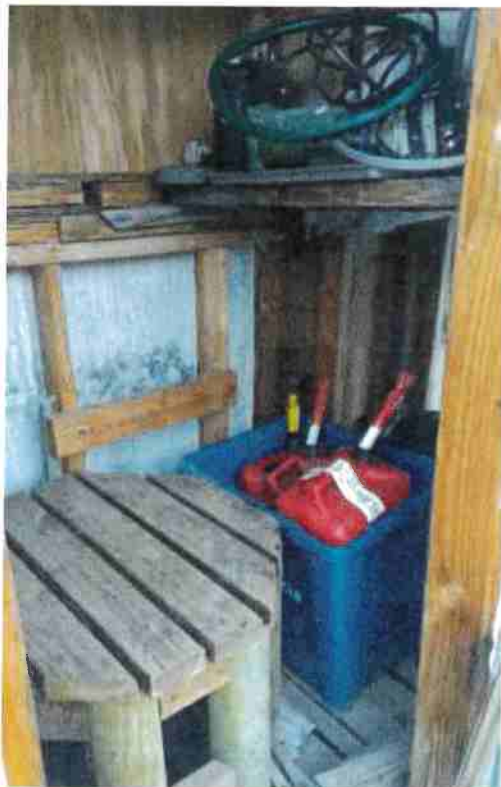
Photo 6. Fuel stored in secondary containment – 2/13/18
