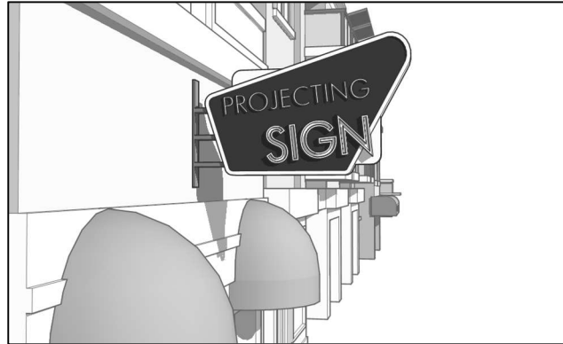
Figure 340-11: Projecting and Suspended Signs
