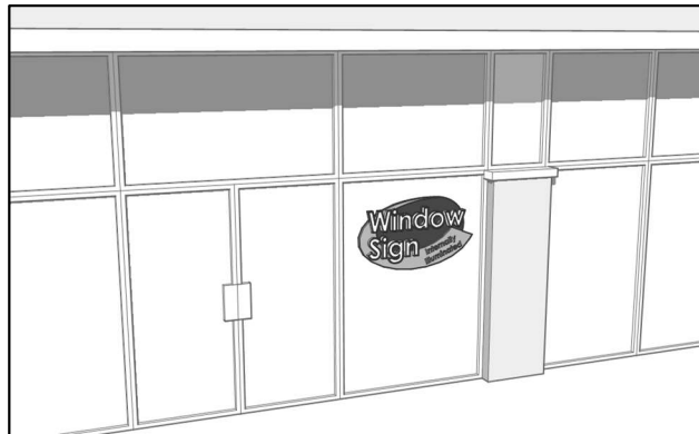
Figure 340-10: Window Signs, Internally Illuminated
