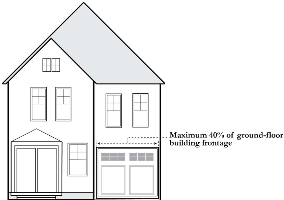
Figure 312-5: Maximum Garage Door Width
