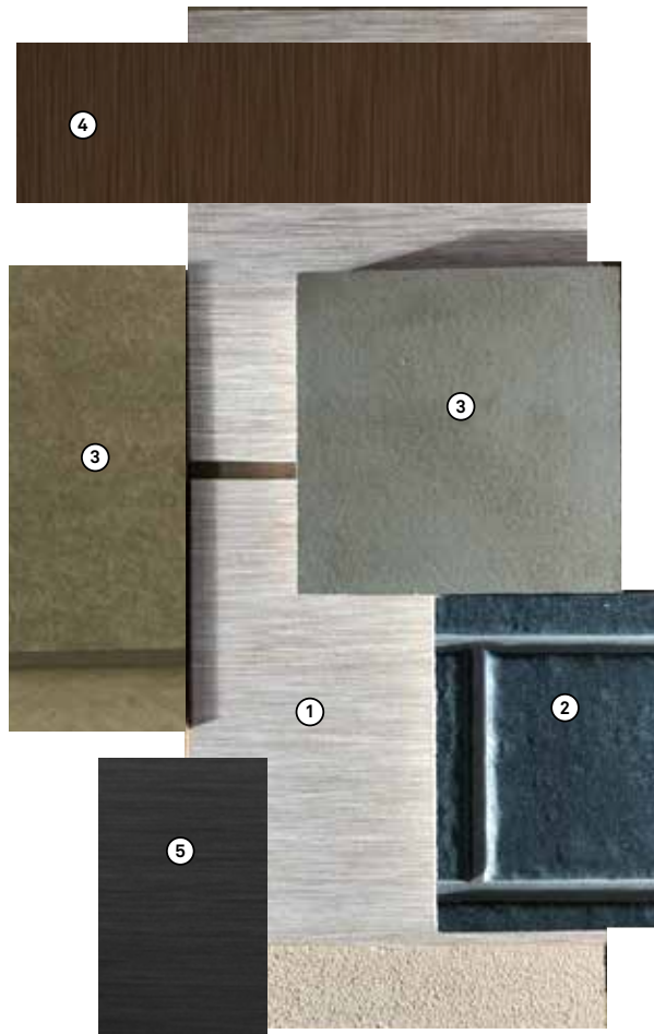
Exhibit B - Materials for 236 G Street. 1. Modern Mill woodless shiplap siding, 2. v Cement Board 3. Hardie V-Groove Trim 4. Bronze Detail 5. Gunmetal Black detail.
