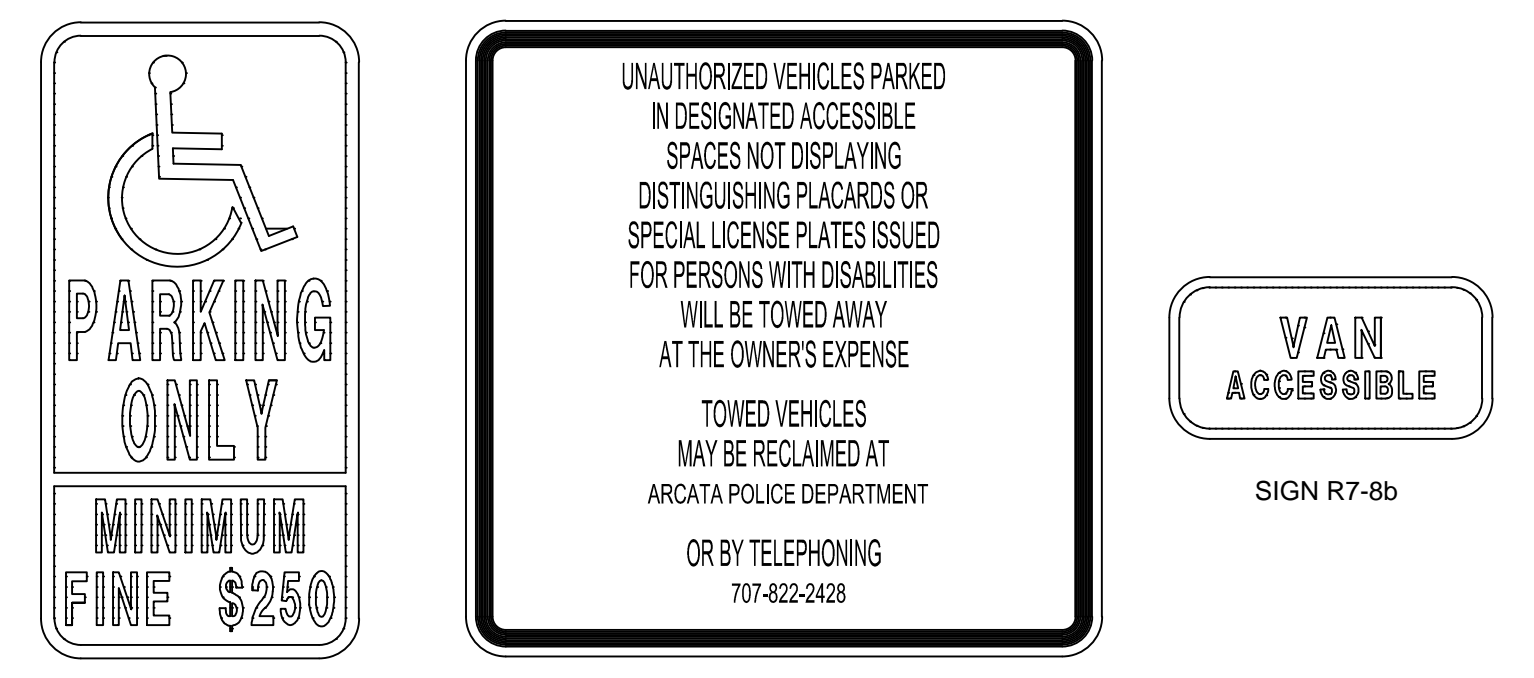
3 ACCESSIBLE PARKING SIGNS SCALE: NTS
