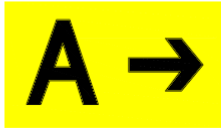
Direction/Runway Exit Sign
