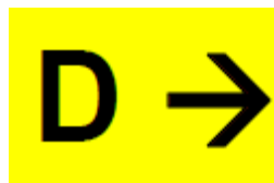
Taxiway Direction Sign
