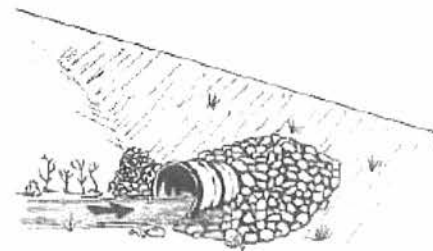
FIGURE 107B. Riprap armor at culvert inlet (Keller and Shear, 2003).
