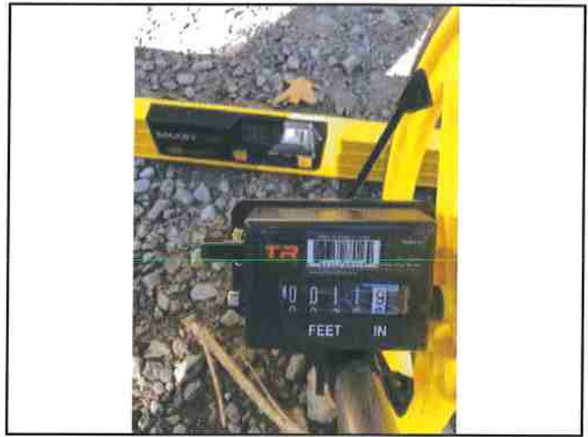
Photo #374 River Rd Slope 19.0% Width 11.9'
