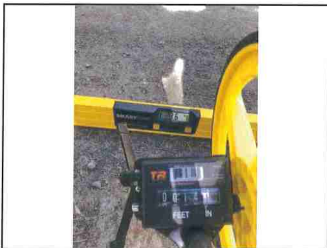
Photo #131 River Rd Slope 3.6% Width 14.1'
