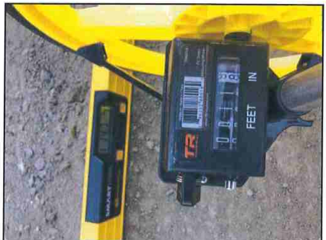
Photo #394 River Rd Slope 14.7% Width 11.8'
