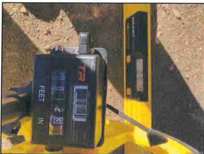
Photo #413 River Rd Slope 0.9% Width 12.3'
