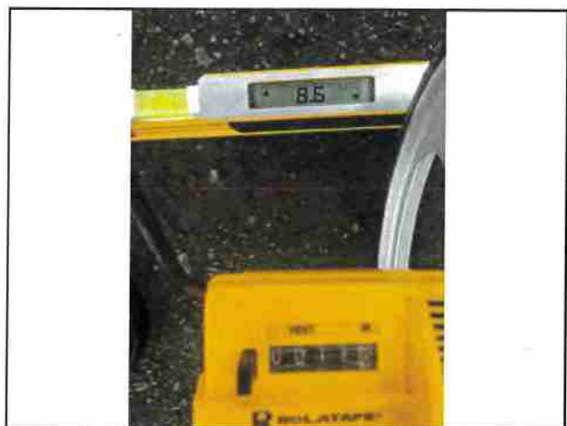
Photo #84 Private Access Rd Slope 8.6% Width 11'9"
