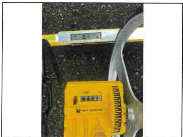
Photo #60 Private Access Rd Slope 8.4% Width 12'0"
