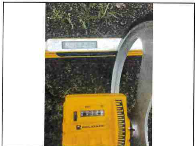
Photo #36 Private Access Rd Slope 16.2% Width 12'1"
