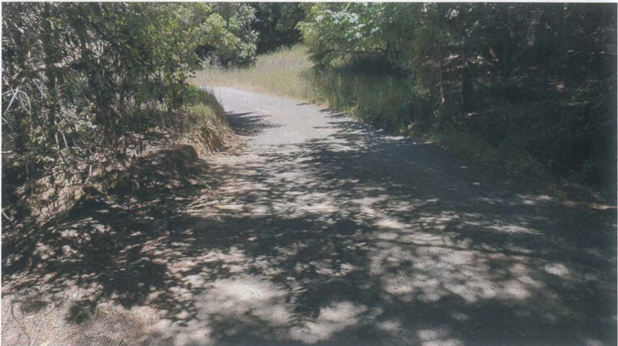
Site 13. Looking up grade at Site 13. A Class III watercourse is diverted down the inside ditch to the right. Re-alignment of this watercourse will consist of a culvert installed diagonally across the road from the grass patch in the upper center-right to the lower left of the photo.
