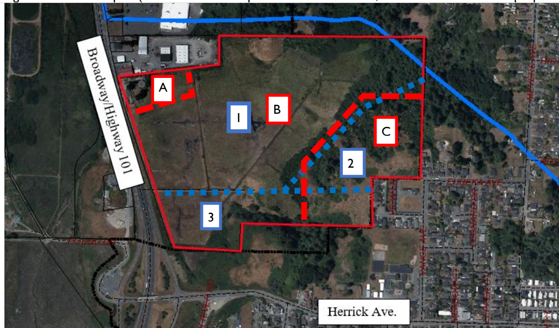
Figure 2: Aerial site plan (blue broken lines represent current lot lines, and red broken lines are proposed)
