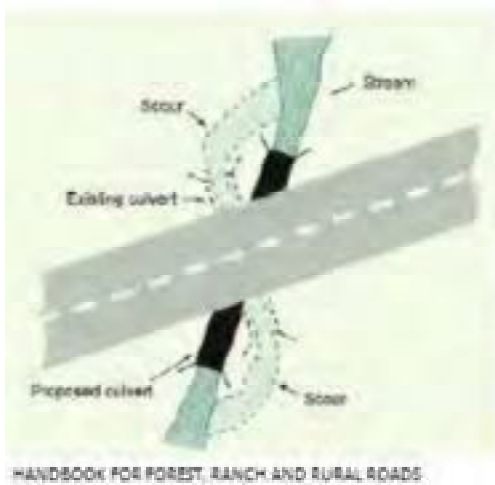
FIGURE 97. Culvert alignment should be in relation to the stream and not the road. It is important that the stream enters and leaves the culvert in a relatively straight horizontal alignment so streamflow does not have to turn to enter the inlet or discharge into a bank as it exits. This figure shows a redesigned culvert installation that replaces the bending alignment that previously existed. Channel turns at the inlet increase plugging potential because wood going through the turn will not align with the inlet. Similarly, channel turns at the inlet and outlet are often accompanied by scour against the channel banks (Wisconsin Transportation Information Center, 2004).
