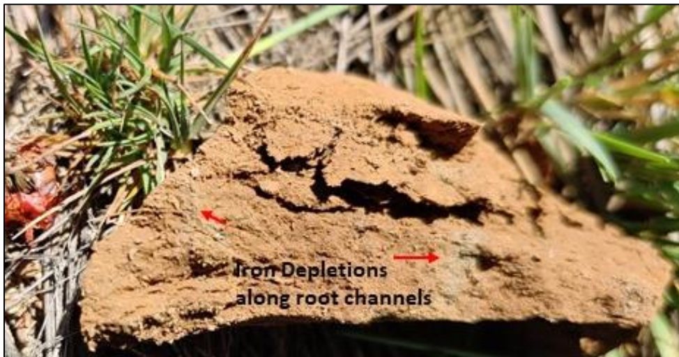
Image 4. Example of iron depletions along root channels. Soil sample is from depressional wetland soil Profile.
