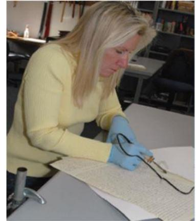
Adhesive reduction begins with the most benign process. If mechanical tape removal is unsuccessful, the next alternative is chemical. This is either a local or spot treatment or immersion in a solvent bath. Kofile ensures that its laboratories are equipped to process chemical treatments correctly and safely. Previous repairs that cannot be removed safely will remain.
