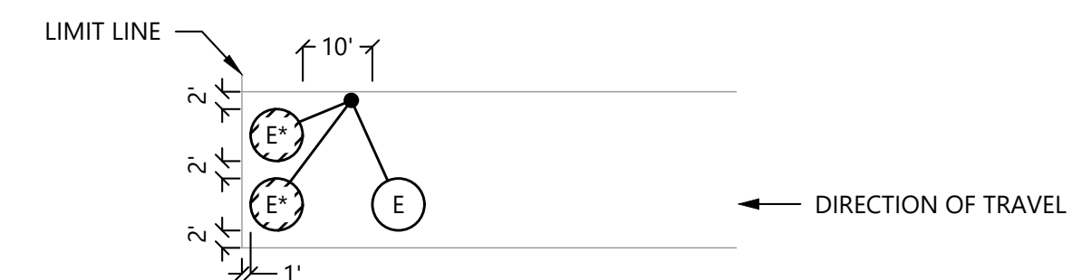
TYPICAL LOOP DETECTOR NOT TO SCALE
