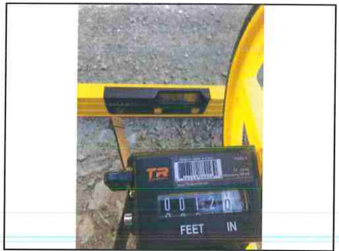
Photo #128 River Rd Slope 14.2% Width 12.0'
