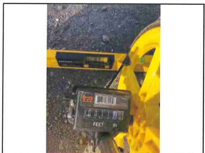
Photo #222 River Rd Slope 8.9% Width 11.7'
