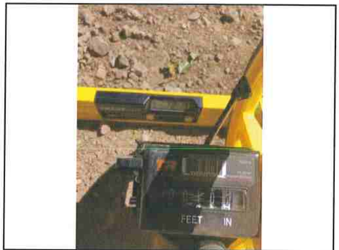
Photo #119 Private Access Rd APN 208-221-014 Slope 21.2% Width 10'10"
