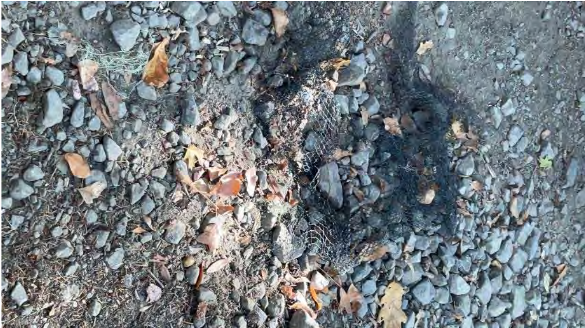
Fig. 11.1 Plastic remnants from old erosion control measures remain on the landscape. Point 11A. Photo by NCRWQCB, 24 October 2024.
