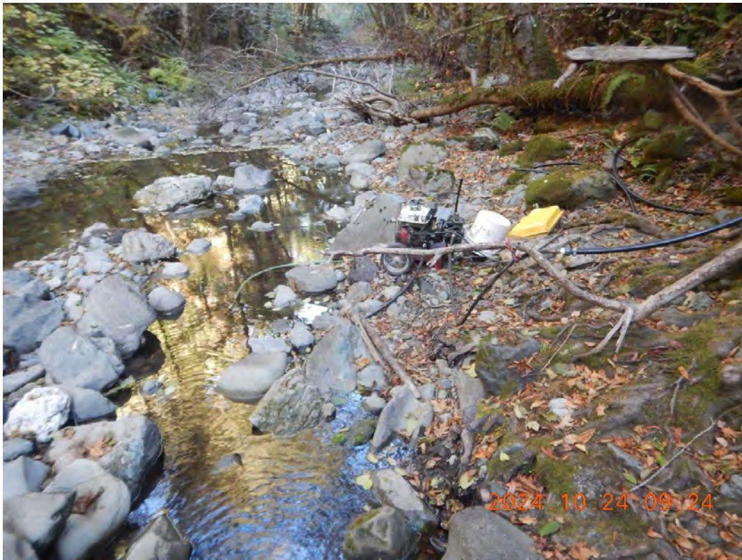
Fig. 2.1 Surface water diversion with gas pump in Little Larabee Creek. Photo by NCRWQCB, 24 October 2024.
