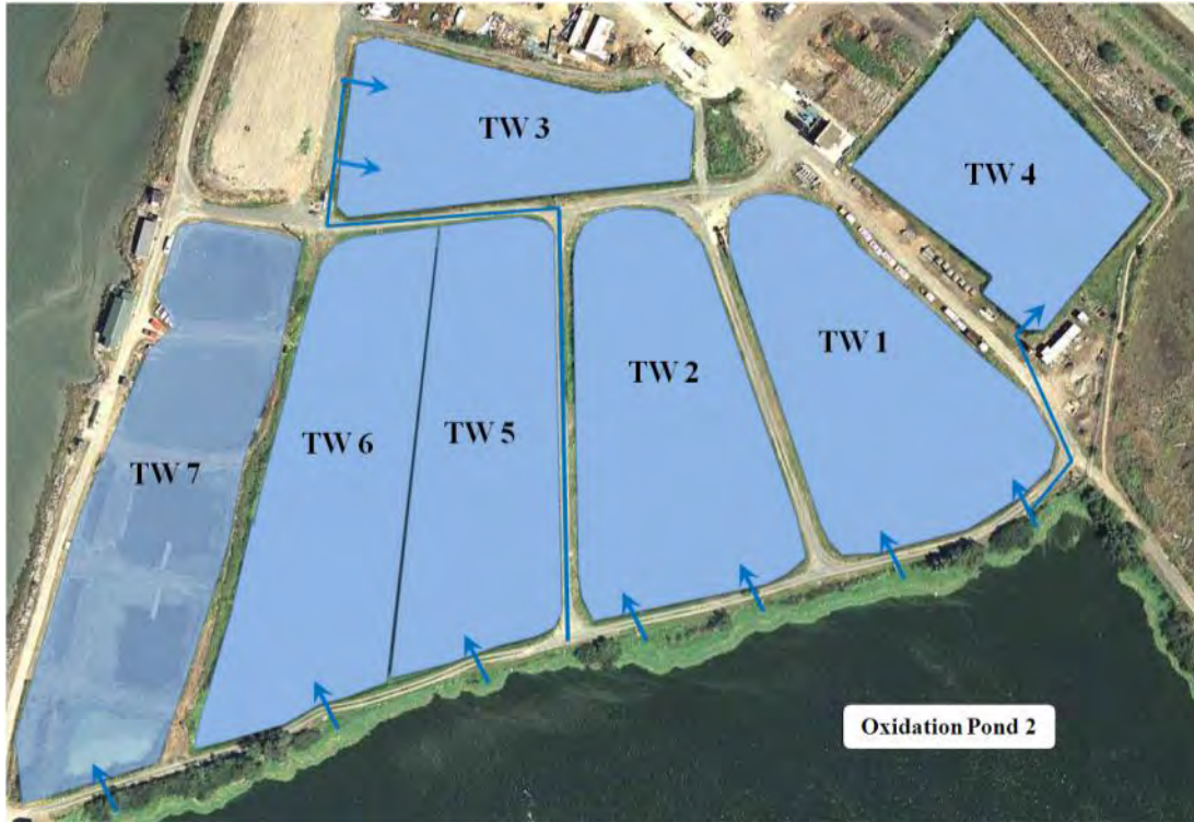
Figure D-4: Treatment Wetlands Site Aerial Showing Influent Weir Configurations
