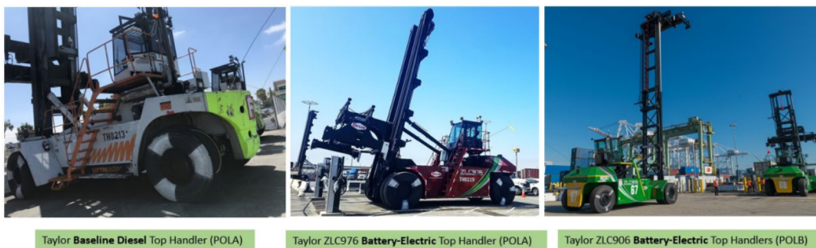
Figure 6. Taylor Machine Works baseline diesel (left), and 2021 prototype ZE top handlers in the Port of Los Angeles (middle) and Port of Long Beach (right). Source: 2021 UPDATE Feasibility Assessment for CHE – Assessment of Commercial Availability.
