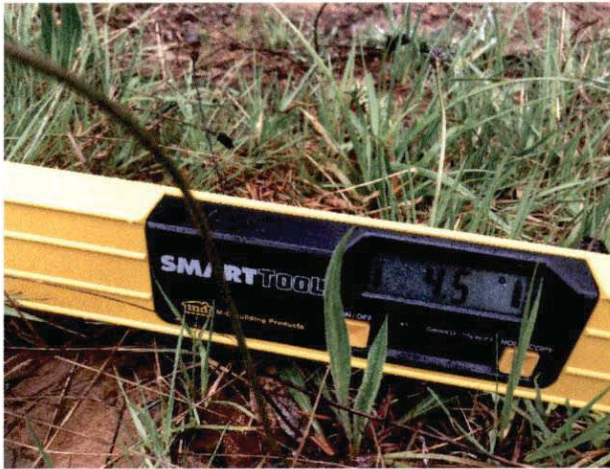
Photo #3 Grade on Access Road
